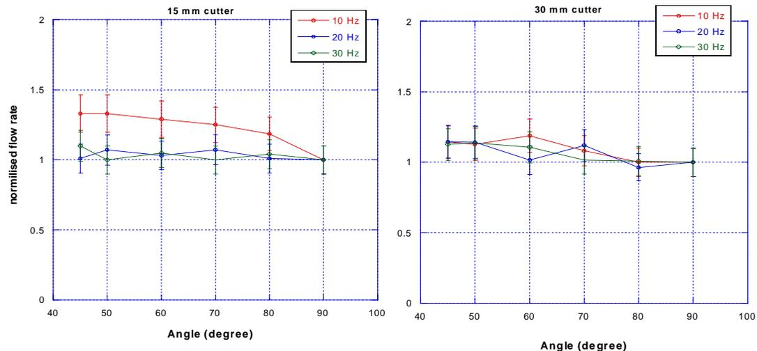
Figure 7a,b Normilised Mass flow rates as a function of inclination a) 15 mm cutter b) 30 mm cutter
