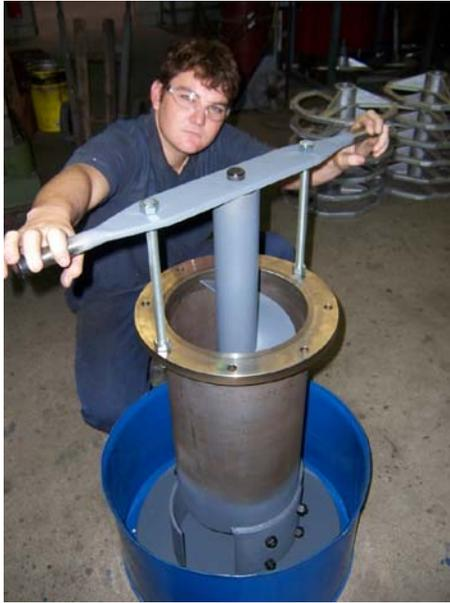
Figure 18 – Empty 254 mm (10”) diameter test elevator.
