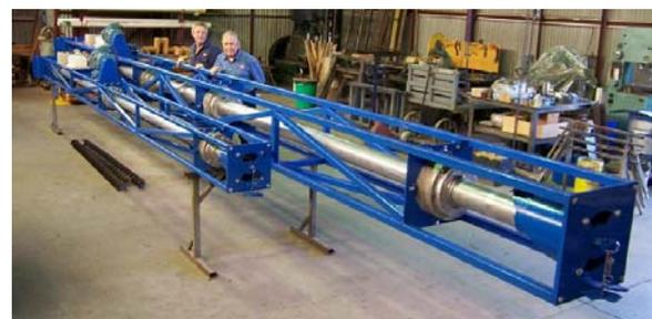
Figure 4 – Completed 100 mm (4") diameter by 7 meters and 152 mm (6") diameter by 10.7 metres lift Olds Elevators for Bean Growers Australia at Olds Engineering, Maryborough.
