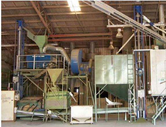
Figure 5 – 150 mm (6”) by 7.5m and 7 m lift Olds Elevators at Bean Growers Australia.
