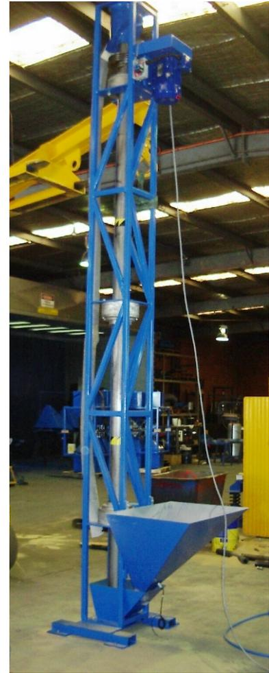
Figure 3 (right) – The elevator being used for lifting sand in a foundry in Singapore.
