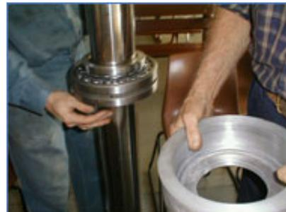
Figure 12 – bearing fitted to elevator, and bearing housing.
