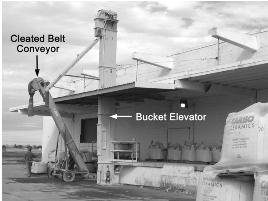
Figure 9 Bucket Elevator and Cleated Belt Conveyor used originally by Carbo Ceramics
